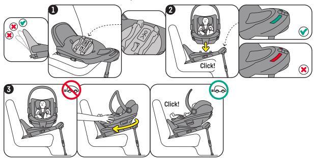
Using the lay-flat function (base installation only)
